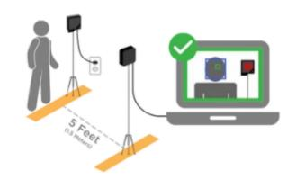
Seek Scan works by preventing fever induced individuals from entering a facility. Set up, the thermal/visible camera and fixed heat source stand across from each other. Standing in front of the camera, the individual's temperature is read, which then notifies the administrator's laptop. No training is required to use Seek Scan.
